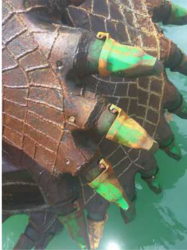
Cutter teeth with new locking pins imported from Netherland
